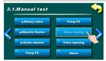
Option for protection valve (closing) test.
