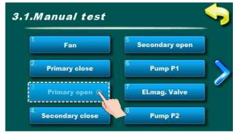
Option for primary air motor device (open direction) test.
