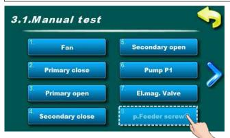
Option for feeder screw test.
