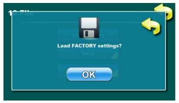
After pressing "LOAD FACTORY" you will see a message "LOAD FACTORY SETTINGS?". Pressing button "OK" will load the default settings of regulation. Pressing the" BACK" will return to the previous menu.
