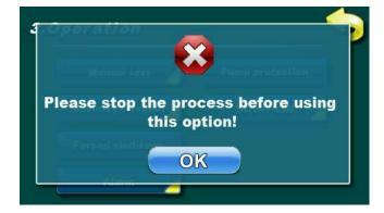
IMPORTANT! To be able to stop all processes, you must first turn off the boiler in the usual way by pressing and then STOP.
