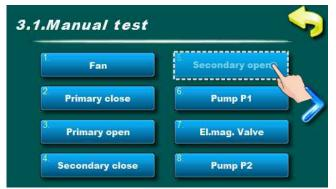
Option for secondary air motor device (open direction) test.
