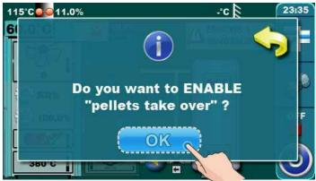
Press green activity indicator on right boiler side (fuel: wood) and hold it for 3 seconds. On display will be desplayed "Do you want to ENABLE "pellets take over?". Confirm it by pressing "Confirm" button.
