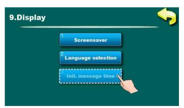
This option is used to set the desired duration of the initial message after turning on the main switch. This option is only available if the option" LANGUAGE SELECTION" (point 9.2.) Is set to "DISABLE".
