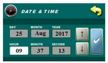
By pressing this option on the main screen you can set the date and time. This option is used to set the date and time. It is necessary for starting times, and the recording of errors/warnings/informations (for the occurrence of errors / warnings, remembers the date and time of occurrence). After setting the date and time it is necessary to press the "CONFIRM" for saving date and time.
