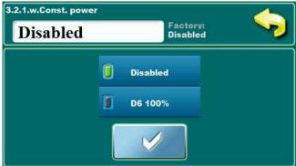
This option allows the flue gas measurement at boiler nominal power (D6).
