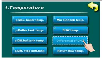
In this parameter is possible to adjust differential for od domestic hot water temperature.
