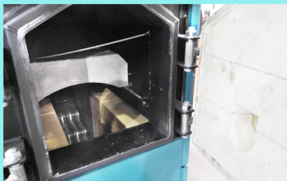
Combustion chamber covered with refractory material and equipped with a moving grate that allows the perfect combustion.
